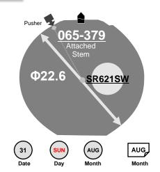
Battery consumption could be minimum by pulling out the stem
